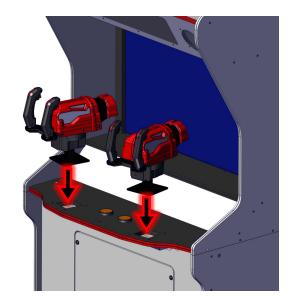
Unpack the two gun assemblies. Insert the gun assembly into the gun mounts on the control panel.
