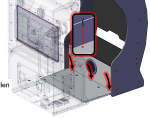
Secure the roof using six AA6220 Allen bolts and six AA6212 washers.
