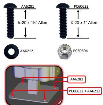
Use PC60622 Allen bolts at the rear and AA6281 Allen bolts with AA6212 washers at the front. Secure the front Allen's with PC60604 nylon nuts.
