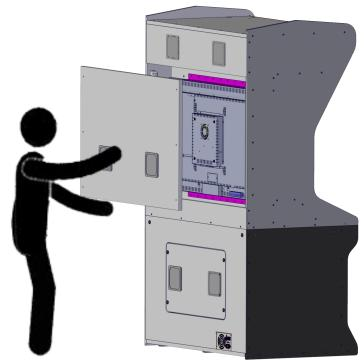
Install one AA6281 Allen bolt and AA6212 washer at each side of the backside of the cabinet. See circle diagrams for locations.
