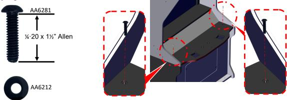
Remove the back panel. There are six AA6220 Allen bolts and AA6212 washers that hold the cabinet back panel on. Put hardware aside.
