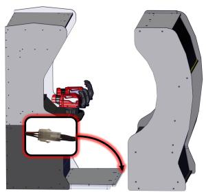
Attach the back harness to the seat assembly.
