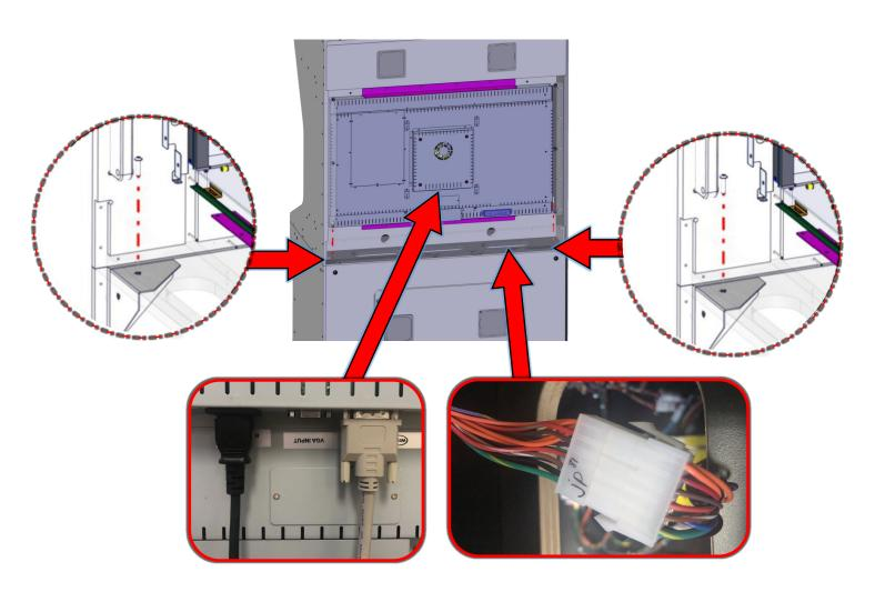
Re-install the back door panel. Use AA6220 bolts and AA6212 washers you removed previously.
